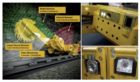
Fig. 4: Environment detection systems on the shearer loader
