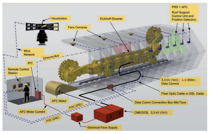
Fig. 5: The shearer loader as a central element in the longwall
